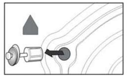
•Unscrew the 4 locking bolts with a spanner. •Remove the rubber and plastic transport brackets from the sockets along with the washers and bolts. •Stop up the holes with the stoppers enclosed in the accessories bag.
